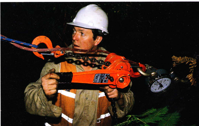
Above: The winch set with the dynamometer 'in line'. The blue rope on the other end of the winch is the prussick loop grasping the red load bearing rope.
